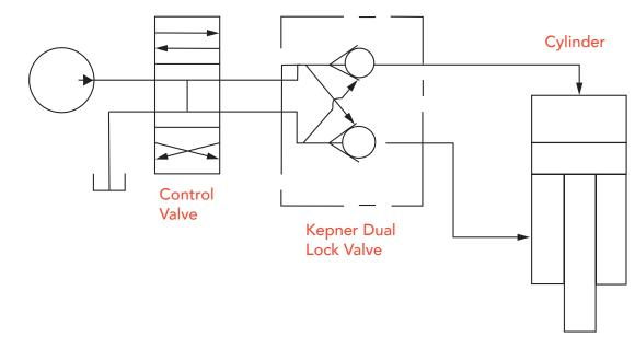
The cylinder piston is locked in place in both directions by the Kep-O-Lok<sup>®</sup> Dual Lock Valve as long as the control valve is centered. When the control valve is shifted to either side, oil pressure on the driving side internally pilots open the other valve module, allowing the piston to move as desired.
